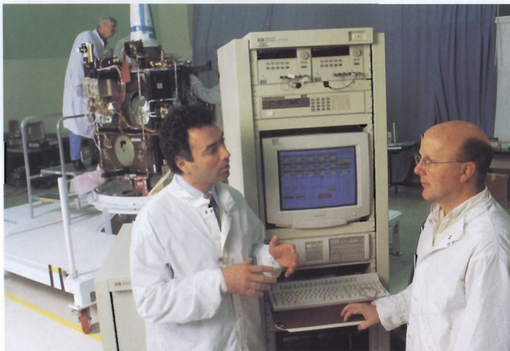
Mark Triolo (left), a solutions specialist from HP's Mountain View, California, office, talks with a Lockheed Martin engineer in front of the HP Electrical Test Set. The customized, off-the-shelf equipment allowed rigorous testing of the craft's electronic structure and payload of sensors and instruments.
